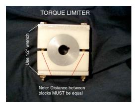
**Note:** If the torque limiter has been slipping excessively, then it may be necessary to undo the two nuts from the bolts and remove the nylon blocks from the mechanism. Sand the blocks as well as the center disk, then replace as shown above.
