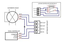
Wiring Diagram for Valve Control, Swap White and Red Wires to Reverse Control Operation
