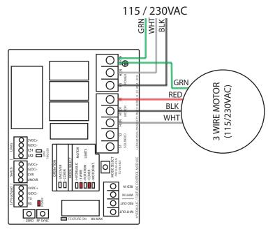
**3 WIRE MOTOR WIRING SCHEMATIC**
