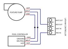
Wiring Diagram for Pump Interrupt 8 Amps or 1/3HP MAX RATING
