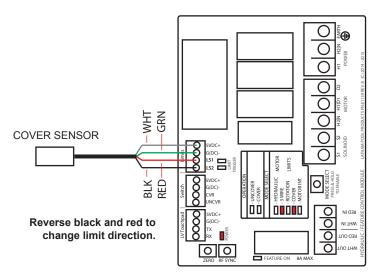
**2013 LIMIT SENSOR WIRING SCHEMATIC**
