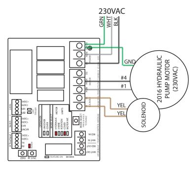
HYDRAULIC WIRING SCHEMATIC
