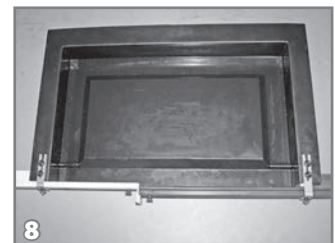
8 Adjust the transition forms side to side to create the size needed for the motor side and non motor side.
