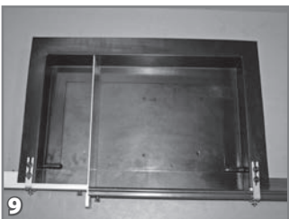
9 Slide the adjustable divider bracket from side to side to create the size of lid section needed.
