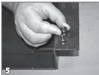
5 Loosely thread the thumb screws into the T nuts that are pressed into the lid form tray.
