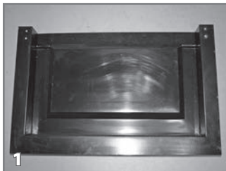
1 Place the lid forming trays on a flat, level surface.
