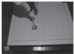
Position the fully assemblied lid panels in the flush deck riser. Use a standard screw driver to twist the lid locks, which will position the lock cam in the slot of the lid lock bracket. This will lock the lid into riser.
