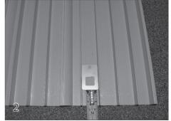
Insert the lid lock backing plate between two ribs on the underside of the lid panel. Position the plate so it is 1-1/4" from the end of the lid panel.
