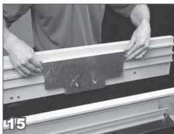
15 Insert the QuickAttach mounting plate over the appropriate anchor plate.
