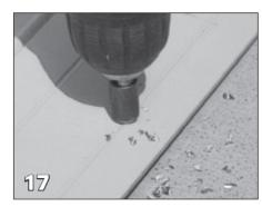
Countersink the drill holes in the hinge.
