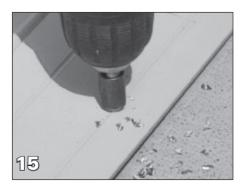
Countersink the drill holes in the hinge.
