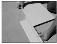
Slide the hinge attachment and lid hinge onto the lid.
