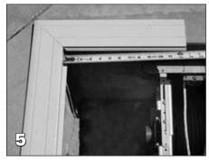
Measure and cut the lid panels (X0048), C-cap (X0053), and hinge attachment (X0940) approximately 1/4in shorter than the actual width to the inside of the lid end supports. This allows the cut cover to attach to the ends of the lid panels to cover any cuts.
