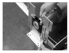
The roll up tube brake should be tight enough to prevent the cover from rolling off the tube faster than it is being pulled into the tracks. To adjust this brake, use two 7/16" wrenches and tightening or loosening the thru bolts in the brake block.
