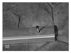
Place the track back over the holes in the deck. Fasten the track screws (19) <u>halfway</u> through the tracks into the plastic anchors. The screws will be fastened completely later in the installation.
