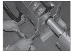
Install the mounting feet on the motor end and non motor end of the mechanism. The height of the mounting feet and the pulley brackets can be adjusted based on the length of the cover to prevent the cover from rubbing on the deck.
