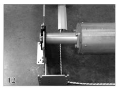
Go to the non-motor end and make sure the rope will come straight back from the rope channel of the track to the pulley. If the ropes do not come straight back, the mechanism should be moved to balance the rope angle on both sides. Only a 1/2" variance from straight is allowed on either side.
