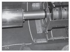
Insert the wire that is attached to the rope into the channel behind the first pulley. Continue to push the wire until it comes out of the channel behind the third pulley.
