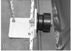
To help the cover roll up evenly, install a cover roller 2-3 inches behind the guide feed. Secure the cover roller to the deck using the screws (19) and anchors (25) provided.
