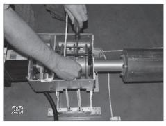
Attaching The Ropes to the Rope Reel Loosen the set screw and remove plastic plug from the rope holder tube. Bring the ropes back to the mechanism. Attach the ropes to the rope reel by inserting the ropes through the center of the rope holding tube and tighten the set screws firmly into the ropes. Some prefer to tie a knot at the end of the rope.
