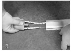
Feed the rope through the end pulley assembly (16) and insert the pulley housing into the end of the track.
