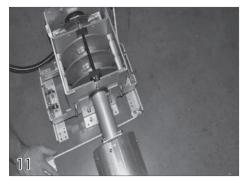
Align the mechanism on the motor side first by using a piece of rope. Extend it from the outside channel of the track to the pulley to make sure the rope will feed directly into the pulley.
