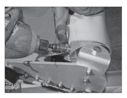
Connect the bonding wire that is attached to the front corner of the cover to the leading edge bar using a tek screw (26). Be sure the screw doesn't interfere with the leading edge insert.
