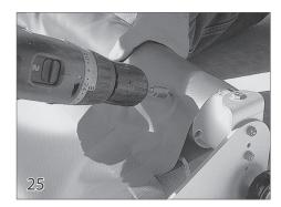
Position the fabric on the leading edge so it is in line with the leading edge support bracket. Secure with a tek screw (26) on the back side of the leading edge. Be sure the screw does not interfere with the leading edge insert.
