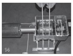
Pull the rope over the rope reel, under the rope containment bracket and out of the mechanism.
