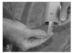
Tap the spring pin (30) into the round splice channel. Slide the center splice (29) into the center channel.
