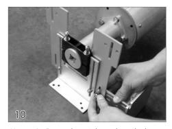
Use a 7/16" wrench to tighten the nylock nuts. Additional carriage bolts (27) and nylock nuts (31) are provided and can be used as reinforcement for the pulley brackets if needed.
