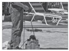
While holding the ropes over the mechanism, run the key switch in the cover position. The excess rope will be wrapped around the rope reel.
