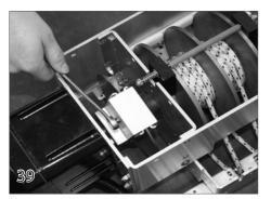
To adjust the torque limiter, use a 9/16" wrench to tighten the first torque limiter bolt 1/2 turn. Run the cover.
