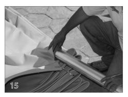
Attaching The Cover Leading Edge Lay the front of the cover in front of the mechanism. Slide the leading edge through the loop on the front of the cover.
