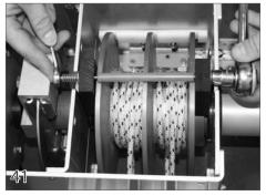
The rope reel brake should be tight enough to prevent the ropes from free spinning off the reel while the cover is opening. If you need to adjust the brakes, use two 7/16" wrenches or sockets to adjust the tension on the rope reel.
