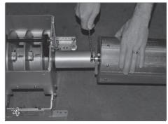
With the motor end turned upside down, attach the cone on the motor end using the same bolts (34) and washers (28). Tighten the bolts using a 9/16" wrench.
