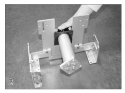
Position the non motor end of the mechanism roughly in the position that it will mounted.
