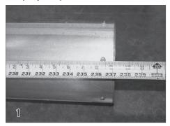
To determine if the cover system was ordered correctly fo the pool, the length of the roll up tube should be 3 inches shorter than the track space.
