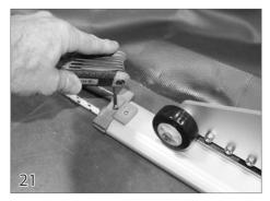
Use a 5/32 allen wrench to tighten the screw that connects the two sections of guide feed together.
