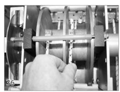
If one of the ropes is longer than the other rope, loosen the set screw that secures the rope to the rope reel lug. Shorten this rope until it is the same length as the other rope. Re-attach the rope to the rope reel.
