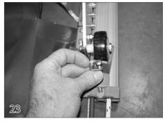
Place a bonding lug (18) on top of the guide feed. Insert a 10-32 x 1 5/8 screw (32) through the lug, guide feed, and track. Install a 10-32 nylock nut (22) and tighten with a 3/8" wrench.
