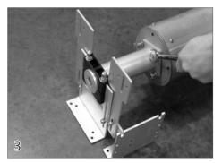
Attaching the Roll-up Tube With the non motor end turned upside down, attach the cone for the non-motor end to the roll-up tube using the 3/8" x 1 1/4" bolts (34) and lock washers (28) provided.
