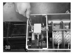
Adjusting The Torque Limiter
