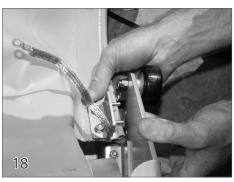
Connect the two hole bracket that is attached to the front corners of the cover to the wheel assemblies.
