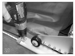
Place a guide feed (15) over the end of the track and drill 3/16 hole through the hole in the guide feed and through the track.
