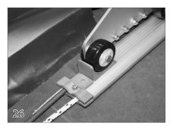
Pull the cover back until the cover is in the track equally on both sides. Pull the ropes tight as they come off the pulleys on the mechanism to eliminate the slack in the rope.
