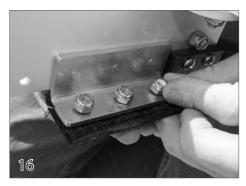
Attach the detachable rope tab to the three hole plate on the wheel assembly.
