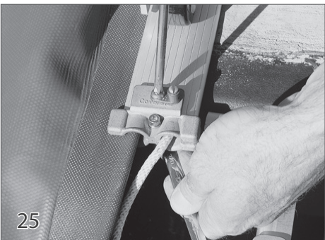
25 Place a bonding wire lug (33) on top of the guide feed and secure with a 10-32 1 3/8" screw (48) and nylock nut (38).
