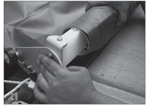
21 Place the nylon leading edge inserts into the ends of the leading edge tube. Make sure they can slide freely inside the leading edge tube.
