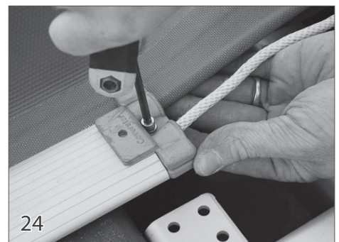
24 Use a 5/32" allen wrench to tighten the screw on the guide feed.
