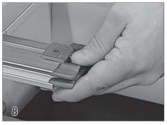
Using a 5/32" allen wrench, loosen the screw on the top of the guide feed (16). Insert the guide feed on the end of the guide that will extend into the housing.
