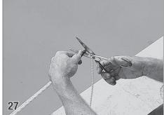
While pulling both ropes tight, use a lighter or torch to burn the ends of the rope. Cut the ropes so they are the same length. **These ropes should be at least 8ft long.** Use a lighter or torch to burn the ends of the rope to keep the rope from fraying. In some cases you will only need to cut one rope.
