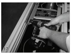
Anchoring The Pulley Brackets Anchor the motor and non-motor end brackets into the housing in as many places as possible.
