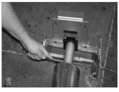
**Connecting the Roll-up Tube** With the non motor end turned upside down, attach the cone for the non-motor end to the roll-up tube using the 3/8" x 1 1/4" bolts (36) and lock washers (37) provided.
