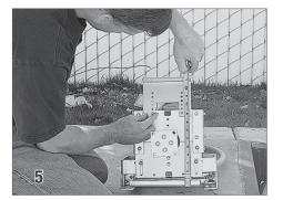
Position the mechanism with the pulley brackets on the bottom. Install the feet on the mechanism using the carriage bolts (35) and nylock nuts (40) provided. Install the feet so the top of the mechanism will be flush with the top of the encapsulation.
