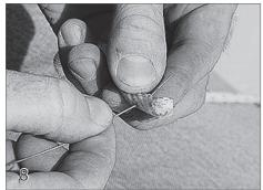
Alternate Rope Feeding Method Another common method of running rope in the track is to pierce the rope with a small piece of wire. This wire then becomes the pulling handle as you feed the rope into the end of the track. This is especially useful if encapsulation isn't being used and the tracks are already installed.
