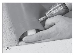
Position the fabric on the leading edge so it is in line with the leading edge support bracket. Secure with a 10 x 1/2" tek screw (31) on the back side of the leading edge tube. Be sure the screw does not interfere with the leading edge insert. Do this for both sides of the cover.
