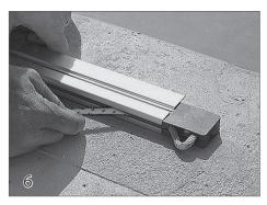
Feed the rope through the pulley (15) assembly. Insert the pulley with the rope onto the end of the track.
