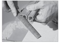
Before splicing the sections of track together, file all track ends thoroughly, rounding all edges and removing all burrs. Clean metal shavings from the track. This step is extremely important! If the track isn't filed smooth, damage can occur to the ropes, slider and cover.
