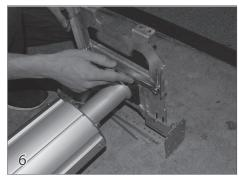
Install the mounting feet on the non motor end using the bolts (47) and lock washers (48) provided. The top of the pulley bracket on the non motor end should be flush with the top of the track.
