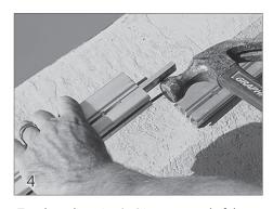
Tap the splice pins (39) into one end of the track and slide the center splice (24) into the center channel.
