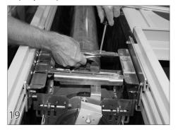
On the motor <u>and</u> non-motor side, use the half inch screws (27) and nylock nuts (29) provided and secure the cross braces together.
