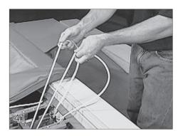
If both ropes are the same length, and the cover doesn't close squarely, shorten the rope for the side of the cover that doesn't close all the way. The amount that the rope is shortened is equal to the distance that the cover needed to travel to close all the way. After shortening the rope, run the switch in the cover position while holding the ropes.
