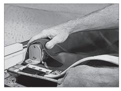
Pull the rope where it comes out of the track as you feed the slider and cover into the track. Keep pulling until the slider is in the track completely.
