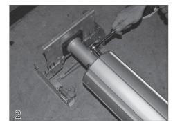
Connecting the Roll-up tube With the non-motor end turned upside down, attach the cone for the non-motor end to the roll-up tube using the 3/8" x 1-1/4" bolts (36) and lock washers (37) provided.
