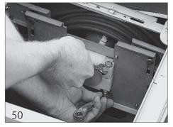
The non-motor brake should be tight enough to prevent the cover from rolling off the tube faster than it is being pulled into the track. To adjust this brake, use two 7/16" wrenches to tighten or loosen the thru bolts in the brake block.
