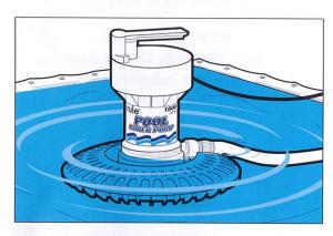
Note: Restricting the flow from a Rule® pump by using a smaller pipe or hose size (such as a garden hose) does not damage the pump, but will result in a reduction in flow. For maximum flow, use the shortest length of the largest diameter hose available.
